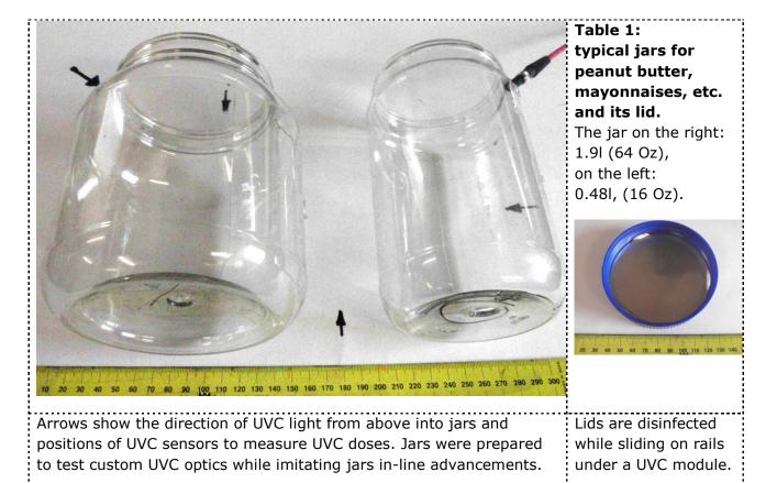
The maximum speeds can be reached for simplest cases of disinfecting from common E-coli, Salmonella and Listeria at 3 to 4 logs (99.9% to 99.99% reduction). De-activating common spores requires higher UVC doses, see Table 2 below. Respective equipment is possible to construct as custom-made.
