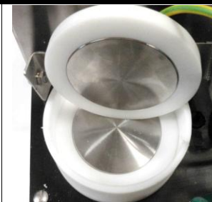
PEF cell with parallel electrodes:
